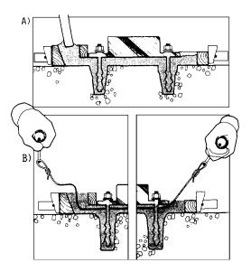
Diagram A illustrates the use of grout surcharge to ensure complete filling under a base.
